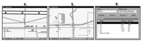
Route creation sequence, continued: (Fig. 4) Point (3) set at on-ramp. (Fig. 5) Waypoint (4) set at highway exit to frontage road leading to river. Waypoint (5) ends the route at a tree stand in a hunting area. (Fig. 6) Press EXIT to save the route and you return to this screen.
